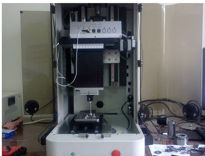
Fig. 1 – The Tribometer CETR UMT 2 with the cylindrical object attached on the pin.
